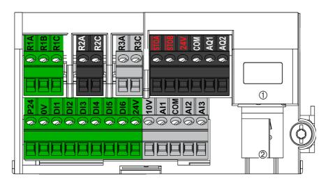
1 Ethernet Modbus TCP, 2 Serial Modbus
