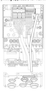
**NOTE:** Cabling plate shown is for frame size 2. Other cabling plates look slightly differs from this one. **NOTE:** For Floor standing products route the control wires into the integrated control cable conduit.
