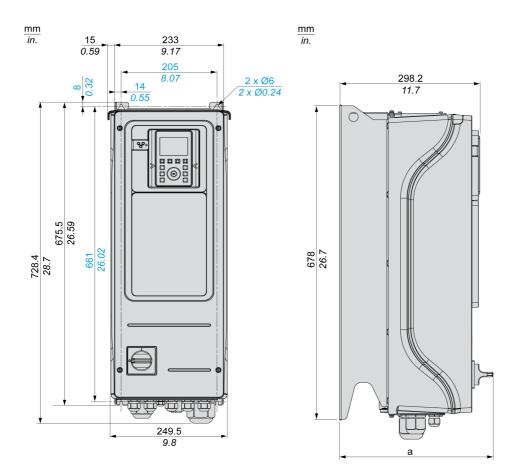
IP55 / UL Type 1 Drives With Load Switch - Front and Side View
