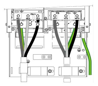
**NOTE:** PA/+ and PC/- terminals are used only to measure the DC Bus voltage and are not intended to be wired for an external use.
