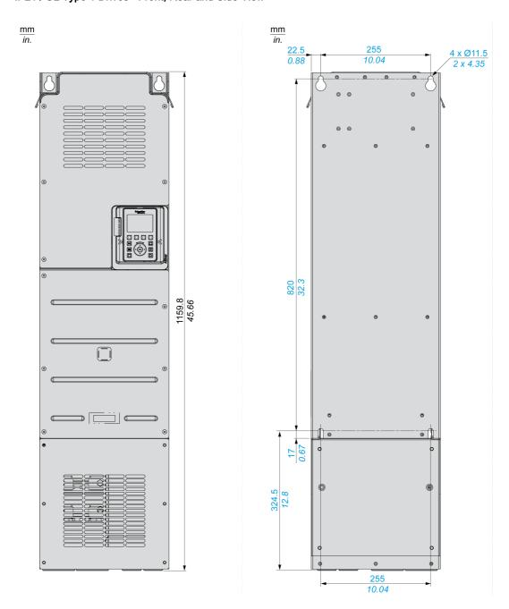
**NOTE:** Lower Conduit Box part sold separately. This part enables wall mounting of the product. It provides IP21 protection degree on the bottom side and UL type 1 protection degree.
