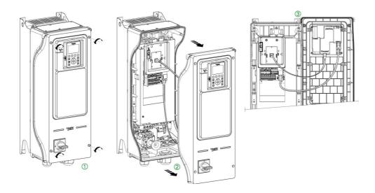
Access To The Terminals For Frame Sizes B and C
