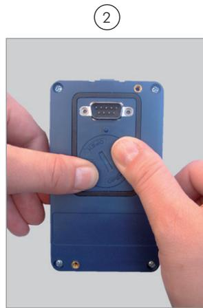
**Press the cover and rotate it counterclockwise**
