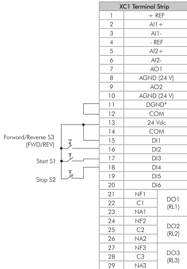
Figure 3.23 - XC1 wiring for control connection 3
