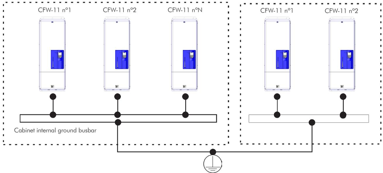
Figure 3.15 - Grounding connections with multiple inverters
