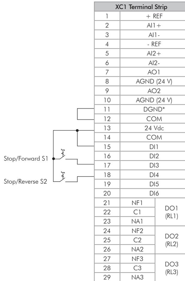
Figure 3.24 - XC1 wiring for control connection 4
