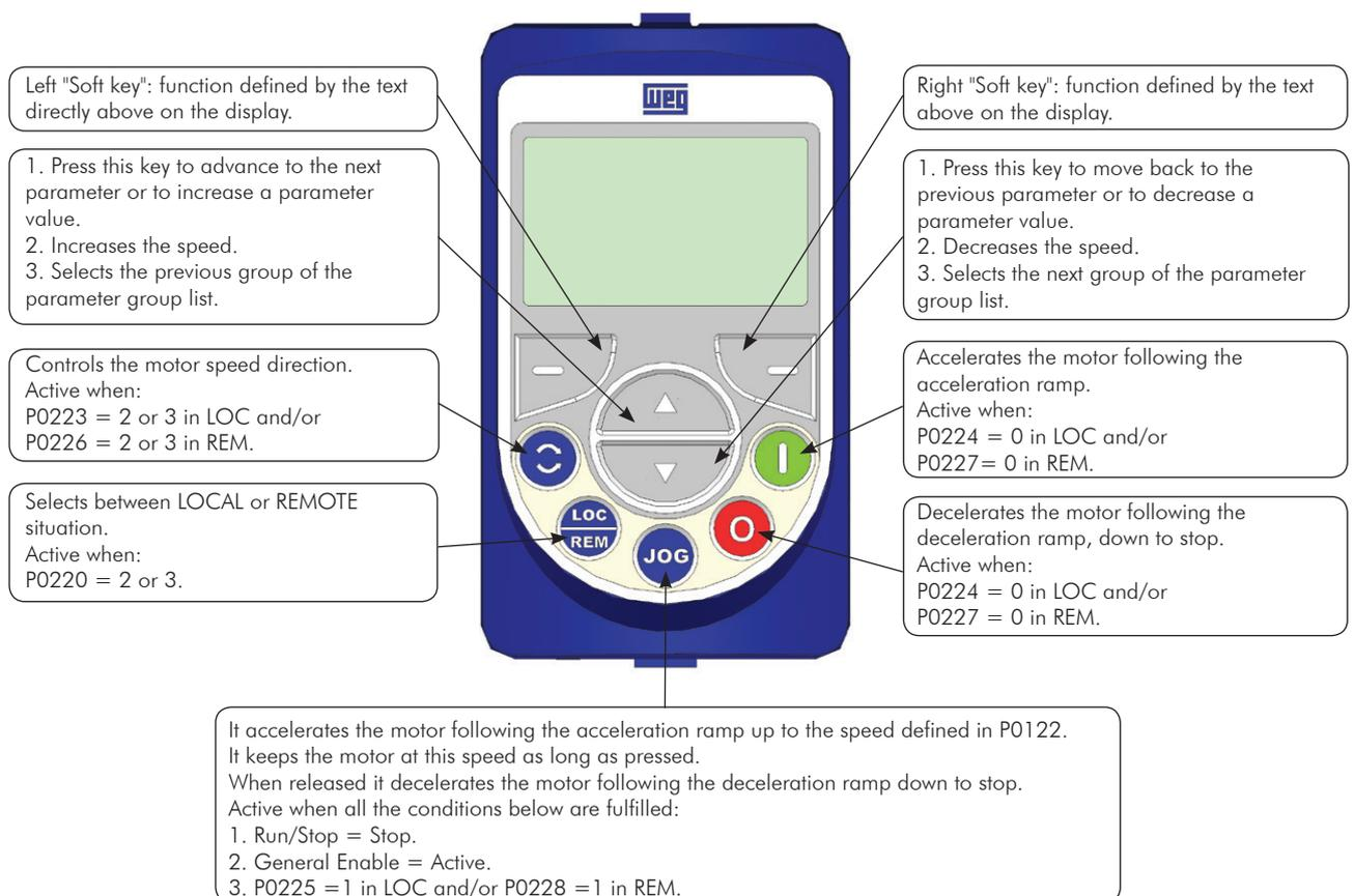
Figure 4.1 - HMI keys
