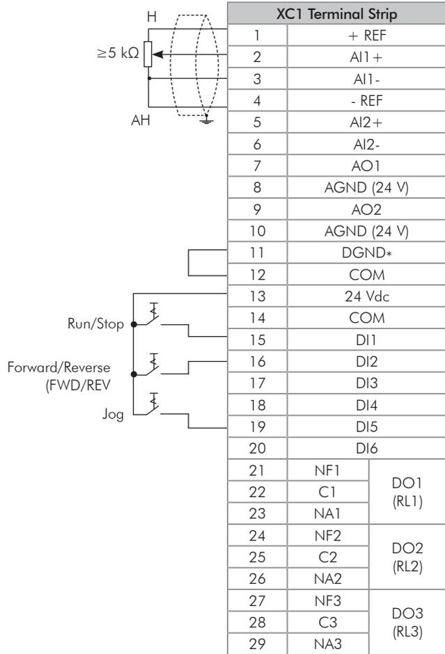
Figure 3.22 - XC1 wiring for control connection 2
