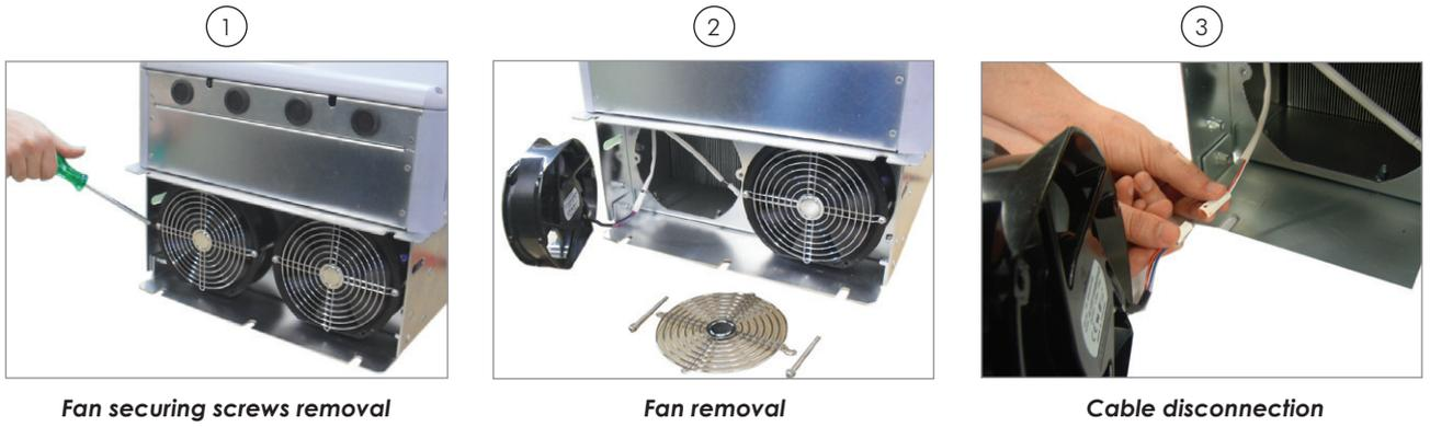
Figure 6.1 - Removal of the heatsink fans
