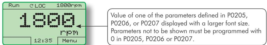
(c) Example of a monitoring screen displaying a parameter with a larger font size
