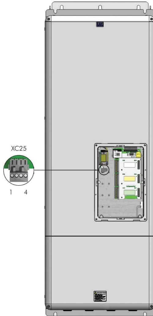
Frame sizes F, G and H inverters - SRB3.00 board
