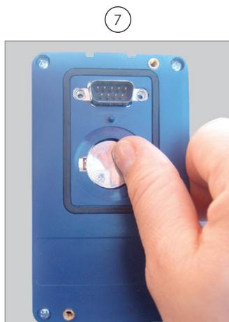
**Press the battery for its insertion**
