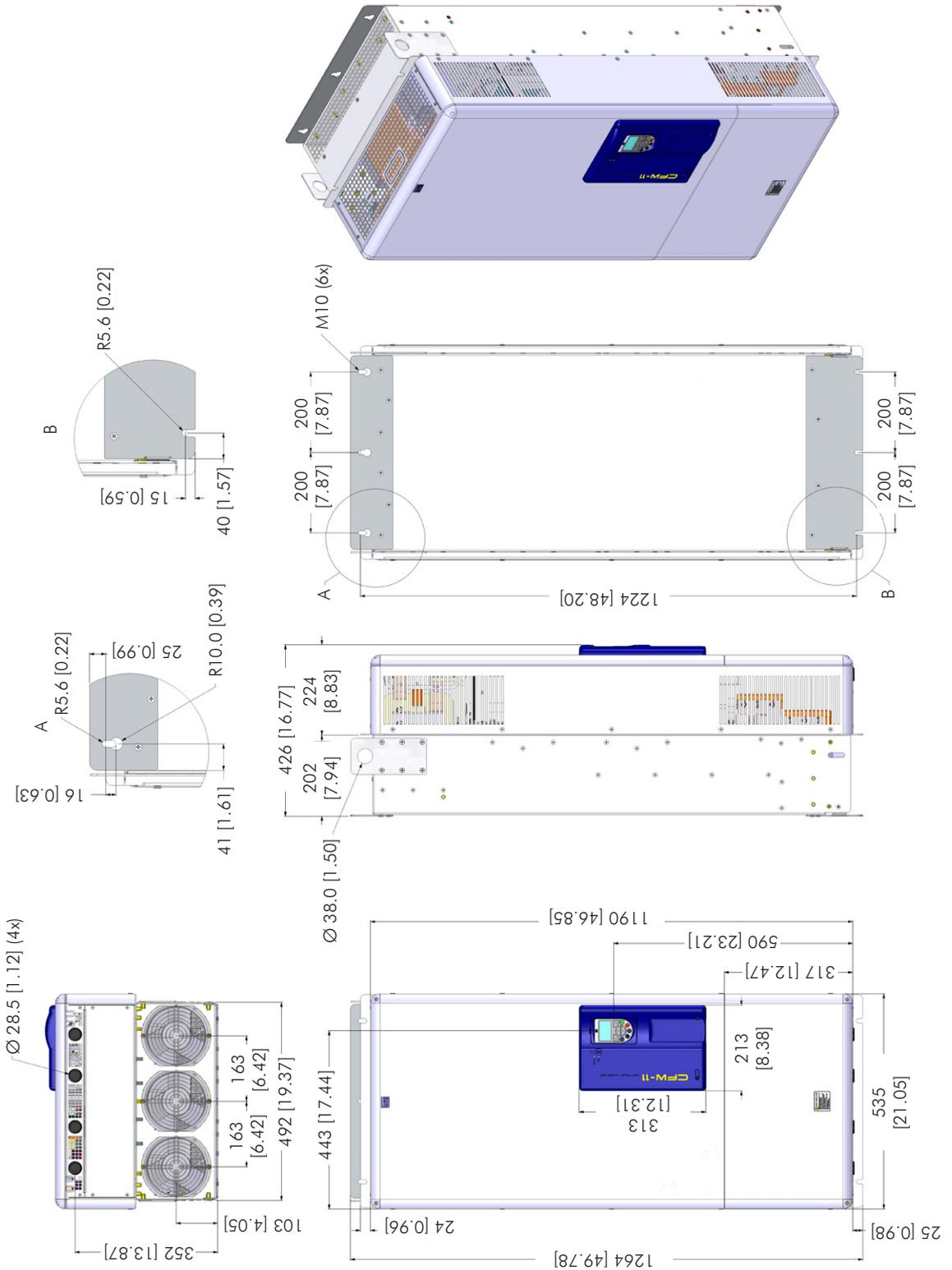
Figure 8.3 - Frame size G dimensions - mm [in]
