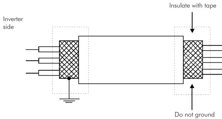
**Figure 3.20** - Shield connection
