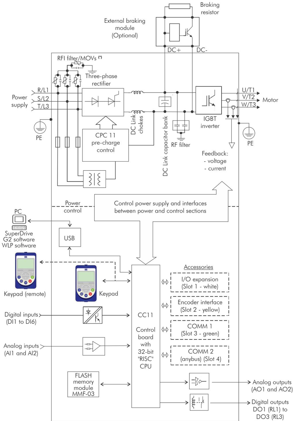
(\*) The capacitor of RFI filter and MOV connected to the ground must be disconnected with IT network, high impedance grounding network and corner-grounded delta networks. Refer to [Item 3.2.3.1.2 IT Networks on page 3-22](#).
