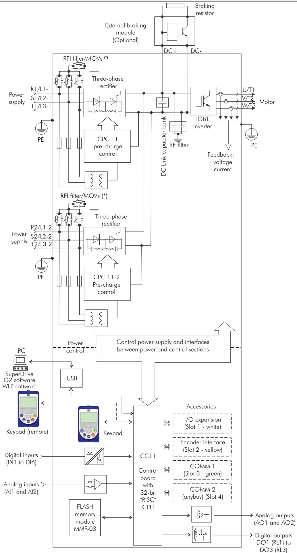
(\*) The capacitor of RFI filter and MOV connected to the ground must be disconnected with IT network, high impedance grounding network and corner-grounded delta networks. Refer to [Item 3.2.3.1.2 IT Networks on page 3-22](#).
