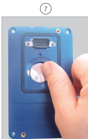
Press the battery for its insertion
