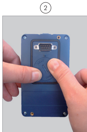
Press the cover and rotate it counterclockwise
